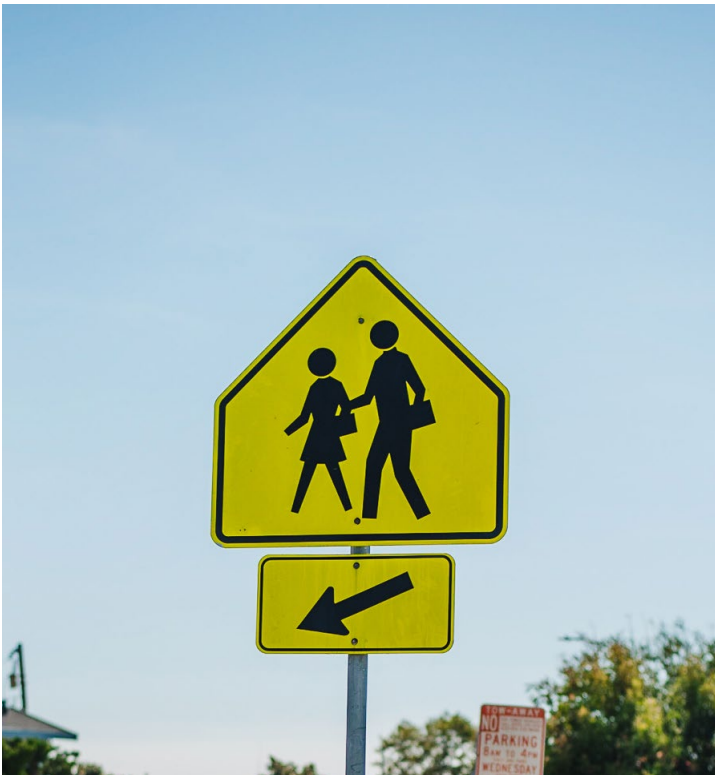
Ensure all school warning signage is updated to current MUTCD standards with fluorescent yellow-green high visibility background.
